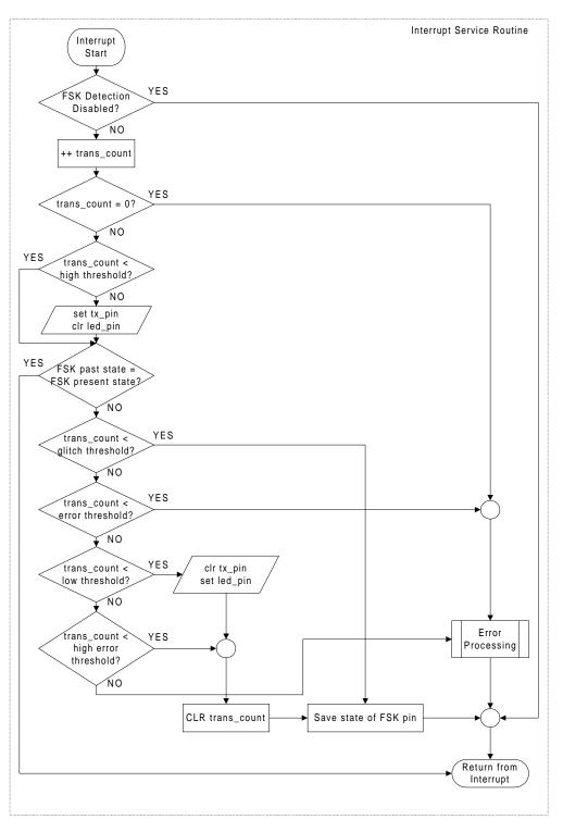
Figure 2-1. Interrupt Service Routine Flowchart
