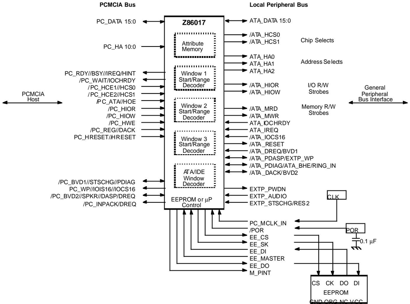
Figure 1-2. Serial Port Master Mode Control
