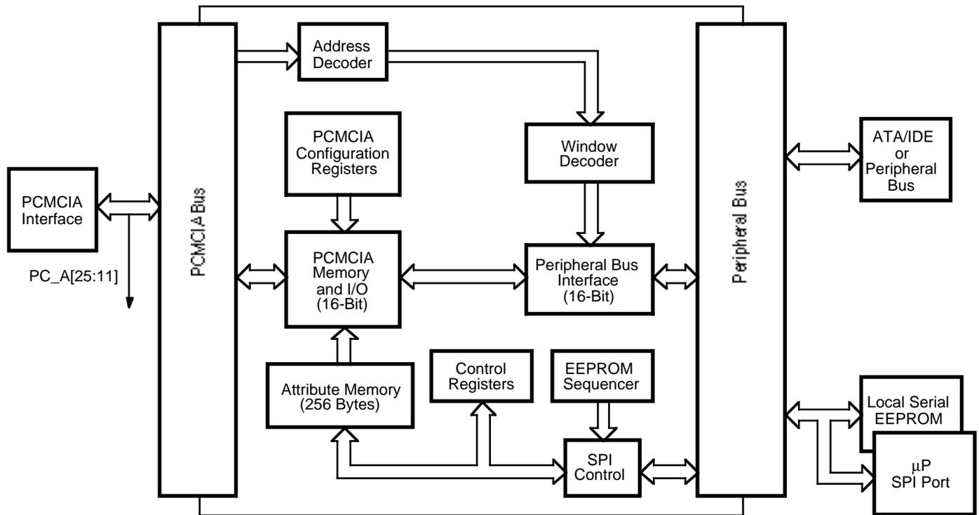
Figure 1-1. 017 Functional Block Diagram
