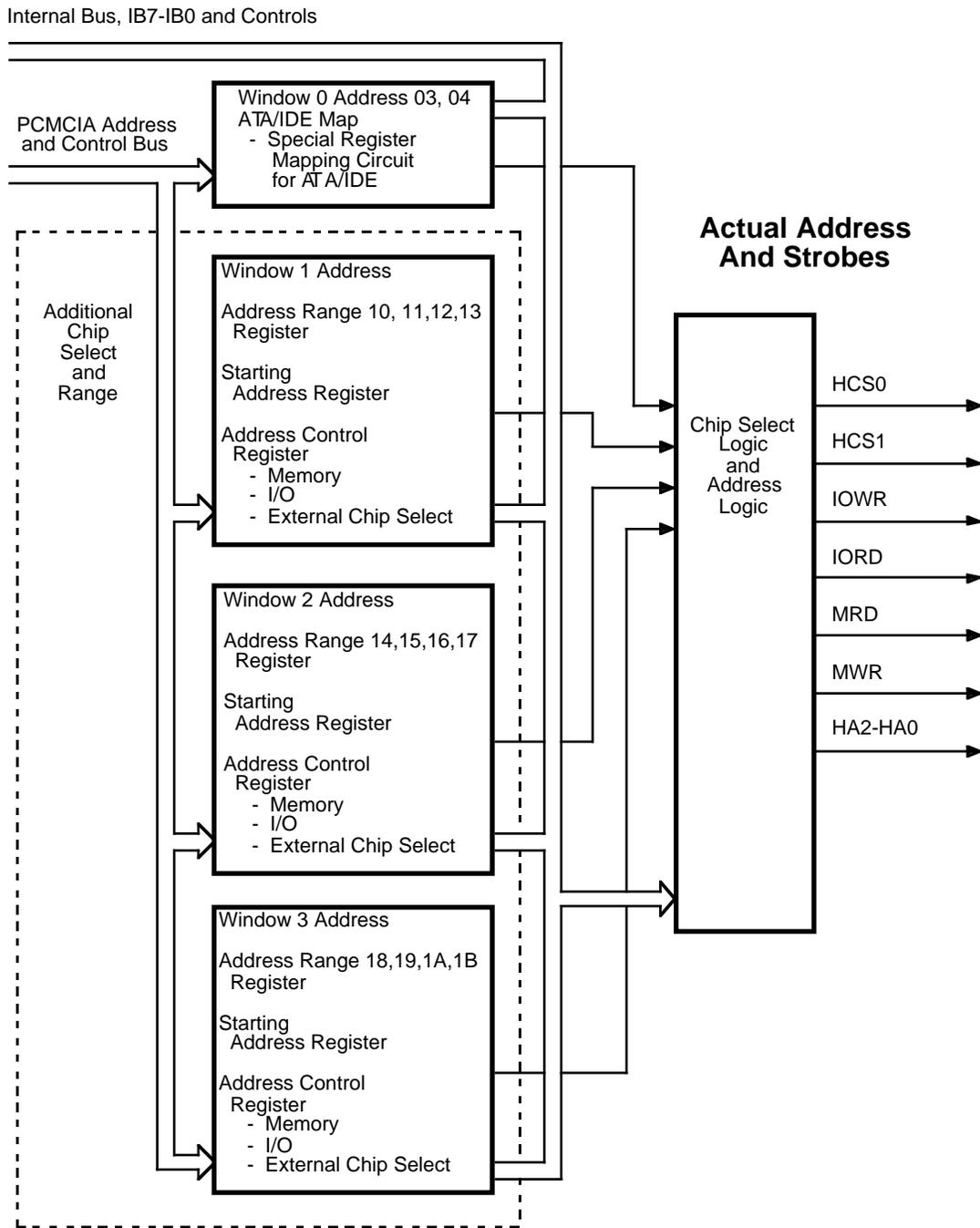
Figure 1-5. Connection Block Diagram
