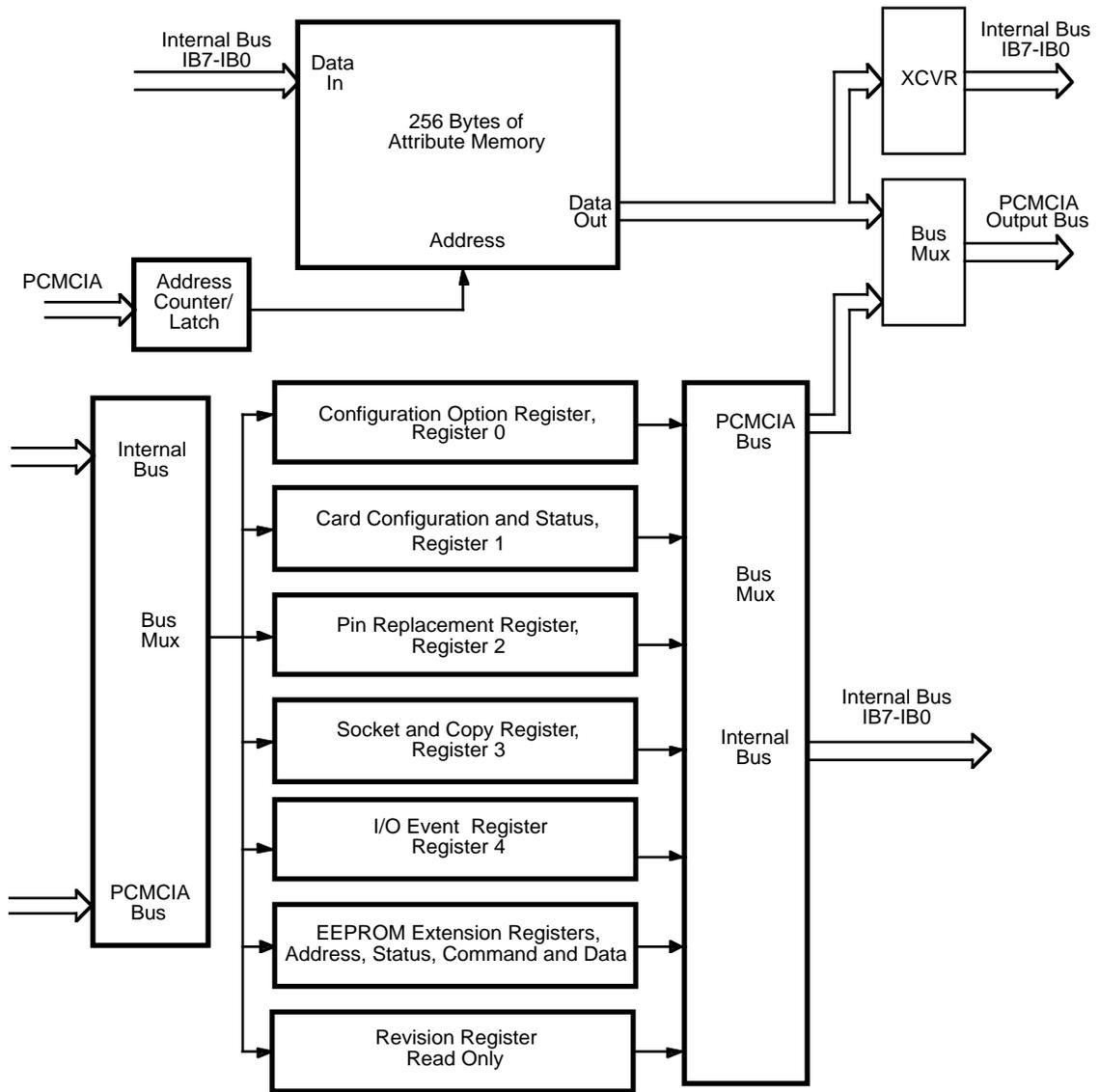
Figure 1-7. Attribute and Configuration Memory Diagram
